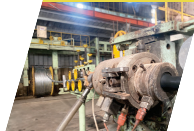
Dây chuyền bọc cáp ngầm FJK 150mm FJK 150mm Extrusion Line for Underground Cable up to 120mm
